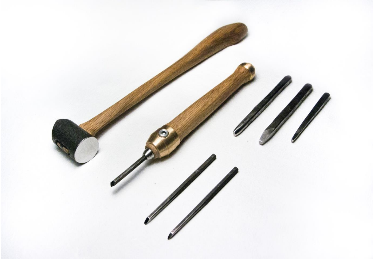
The complete tool kit: oak hammer and engraving tool, three engraving tools and three punches.
